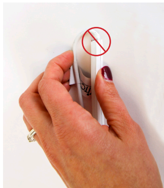
Do not bend right at solder joint
