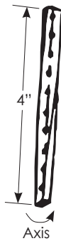
Do not twist more than 90° over the length of one 24V segment / Two 12V segments (4" total length)
